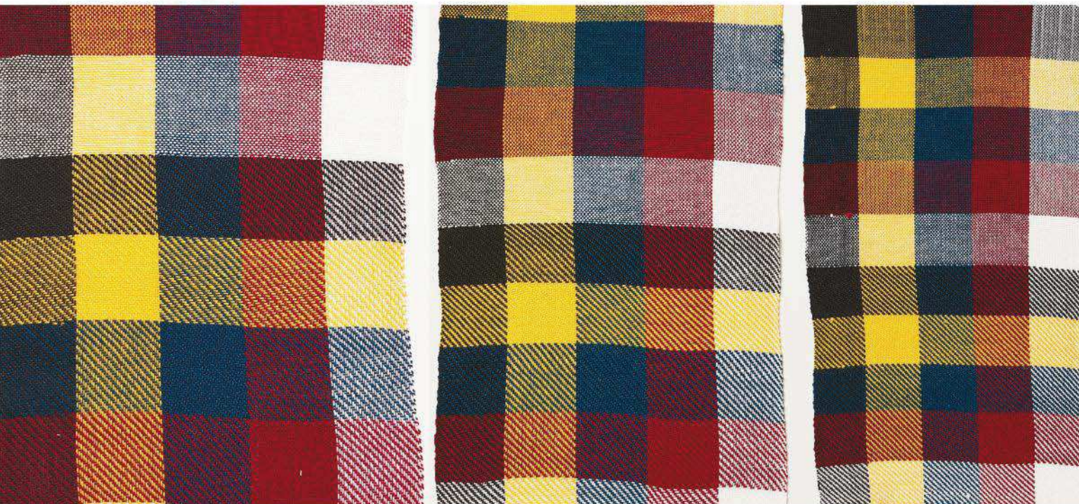
10/2 cotton woven in plain weave and twill sett at 20, 24, and 30 ends per inch (left to right).
