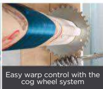
Linen aprons on the cloth and warp beams
